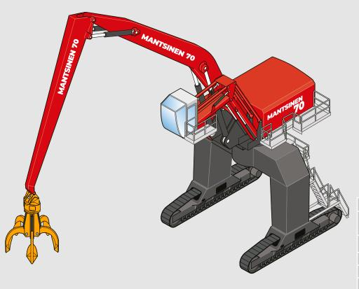
Long and widely extended tracks and rigid box type frame create an excellent and stable foundation for the machine. The flat track shoes run smoothly on gravel, asphalt or concrete. Hydrostatic track drive consists of two speed axial piston travel motors and planetary track drives. The machine is also equipped with spring loaded multi disc automatic brakes with hydraulic release.
