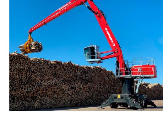
again recovered next lift speeding up the operation. The optional Hybrilift system for Mantsinen 70 is equivalent to 110 hp of engine power at the average lifting speed. It boosts the operation and minimizes energy consumption and emissions accordingly. The system includes temperature compensation providing full lifting capacity also in variating ambient temperatures.
