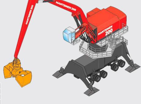
Undercarriages are available in several different heights to optimise the operation, reach and visibility. Mantsinen organization can provide ground pressure information and operational drawings case by case.
