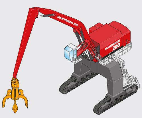
Long and widely apart tracks and rigid box type frame create an excellent stability foundation for the machine. The flat track shoes run smoothly on gravel, asphalt or concrete. Hydrostatic track drive consists of two speed axial piston travel motors and planetary trackdrives. There are spring applied multidisc automatic brakes with hydraulic release.
