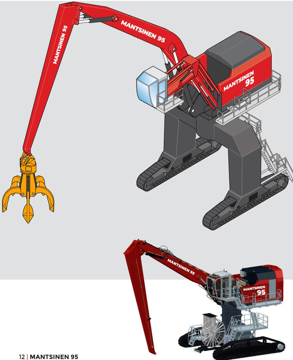
Long and widely spaced tracks and rigid box type frame create an excellent stability foundation for the machine. The flat track shoes run smoothly on gravel, asphalt or concrete. The hydrostatic track drive system consists of two-speed axial piston travel motors and planetary trackdrives. There are spring-applied multidisc automatic brakes with hydraulic release.
